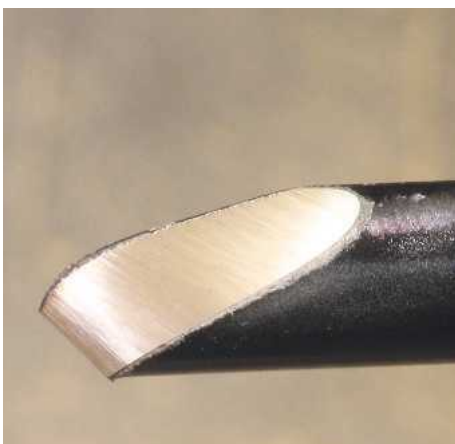
▲ Pic.1 Bowl gouges are measured from the inside of one flute to the outside of the tool, so the 10mm tool is made from 13mm bar, which is a bit confusing! If the tool is ground properly, then the top cutting edge should be straight or slightly convex
